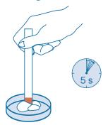
Bring the activated stick into direct contact with the substance to be tested for at least 5 seconds.
