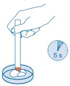
Bring the activated stick into direct contact with the substance to be tested for at least 5 seconds.
